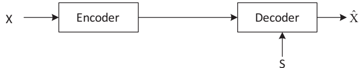
Figure 1: Compression of X when its side information S is available at the decoder
