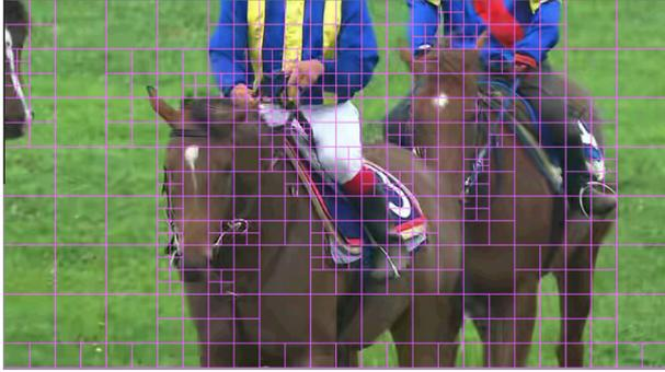
**Fig. 3.** The coding structure for a frame in RaceHorses with HEVC.
