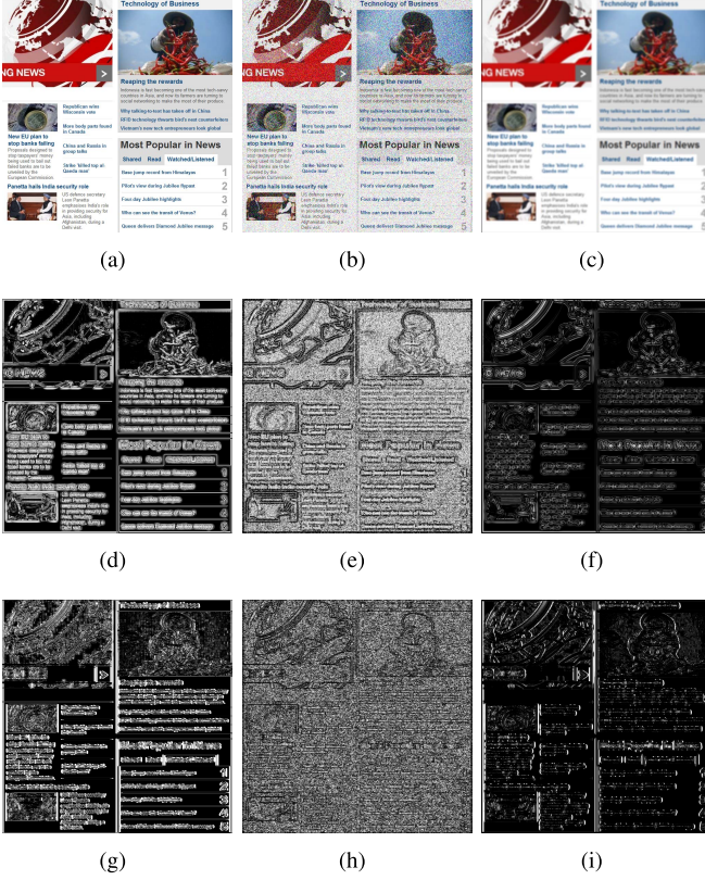
Fig. 5. Illustration of the uncertainty maps from Gaussian blur and motion blur, where the top row shows the SCIs, the middle row shows the corresponding S_G maps, and the bottom row shows the corresponding S_M maps. (a), (d), and (g) Original. (b), (e), and (h) Gaussian noise. (c), (f), and (i) Gaussian blur.
