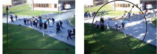
Fig 2 Features are extracted in different coordinate systems. (a) Histograms of orientation and magnitude are computed in 2-D rectangular coordinate system. (b) Histograms of relative orientation ( \alpha ) and relative magnitude ( v ) (referring to O) are computed in polar coordinate system.
