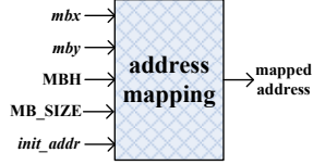
Fig. 8. Block diagram of the address mapping schemes.
