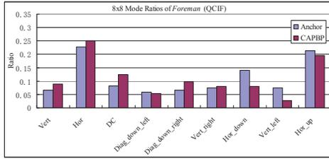
Fig.8 Mode ratio of intra 8x8 block within the first frame of *Foreman* (QCIF@30HZ)
