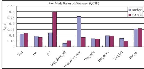
Fig.7 Mode ratio of intra 4x4 block within the first frame of *Foreman* (QCIF@30HZ)
