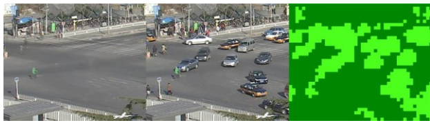
(a)Background frame (b)Current frame (c)BFI Fig.4 The background frame and the classification
