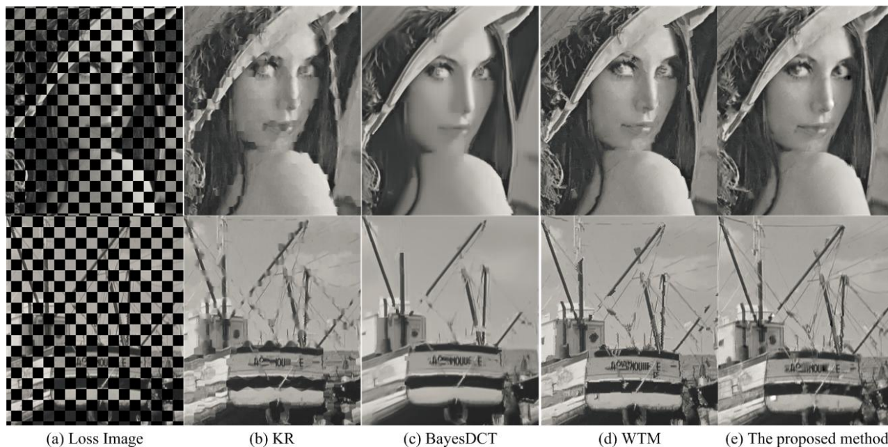
Fig. 2. Objective performance comparison among competing schemes on Lena and Boat with 50% regular block losses
