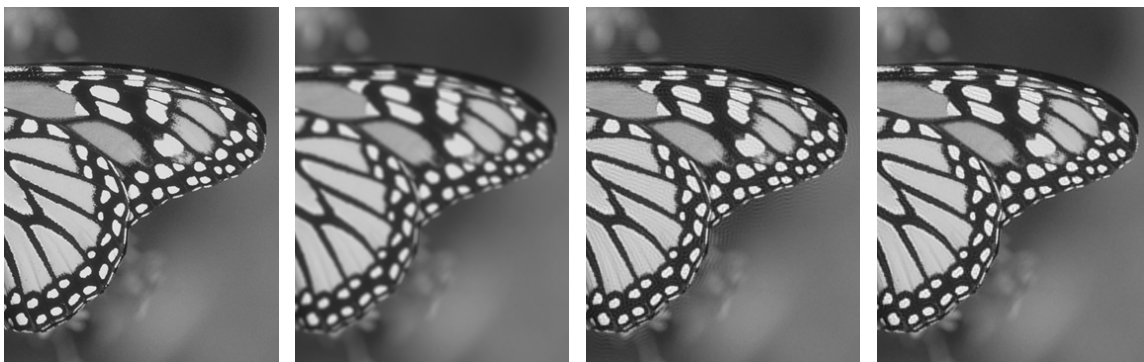
Fig. 1: Evaluation of the proposed method. From left to right: original image (cropped from 512 \times 768 Monarch ), blurred by Gaussian PSF ( \sigma = 2 , 5 \times 5 window), deblurred by iterative back-projection (IBP), deblurred by the proposed method.
