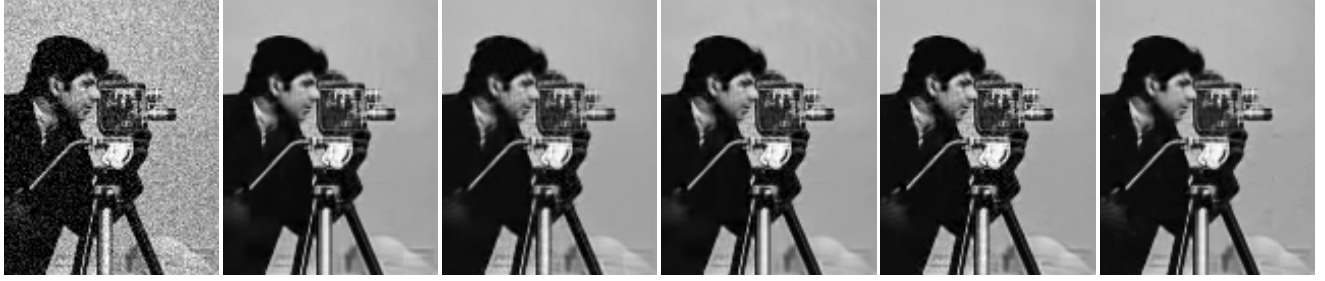
Fig. 1. Denoised fragments of Cameraman . From left to right: (a) Noisy image ( \sigma_n = 20 ); (b) BM3D (PSNR = 30.41dB); (c) LPG-PCA (PSNR = 29.73dB); (d) CSR (PSNR = 30.29dB); (e) LASSC (PSNR = 28.56dB); (f) Proposed (PSNR = 30.66dB ).
