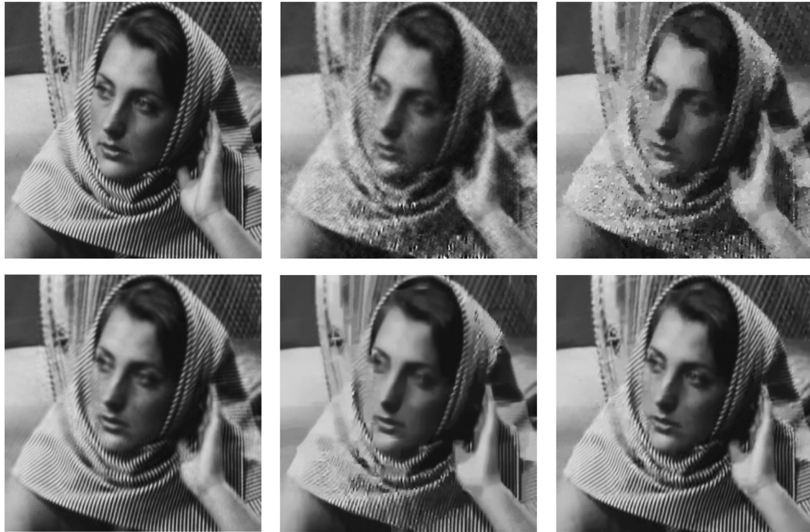
Fig. 7. Visual quality comparison of image CS recovery on gray image Barbara in the case of subrate=20\% . From left to right and top to bottom: original image, the CS recovered images by DWT (PSNR=23.96 dB; FSIM=0.8547), TV (PSNR=23.79 dB; FSIM=0.8199), MH (PSNR=31.09 dB; FSIM=0.9419), CoS (PSNR=26.60 dB; FSIM=0.8742) and the proposed algorithm (PSNR=31.61 dB; FSIM=0.9487).
