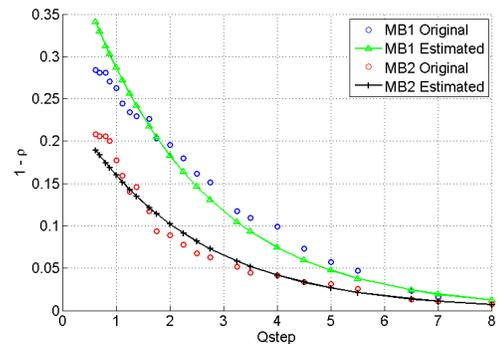
Fig. 2. Relationship between  $1 - \rho$  and  $Qstep$  at the MB level for the Foreman test video sequence (*CIF*, encoded with x264 at 400kbps).
