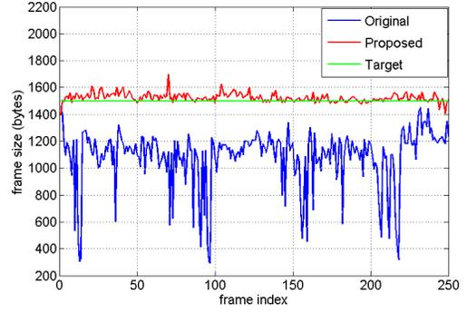
Fig. 4. Bit rate for individual frames for *Foreman* at 300 kbps.
