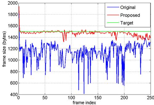
Fig. 3. Bit rate for individual frames for *Football* at 300 kbps.
