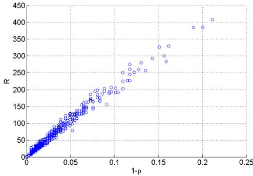
Fig. 1. Relationship between  $R$  and  $1 - \rho$  at the MB level for the Foreman video sequence (*CIF*, encoded with x264 at 400kbps).
