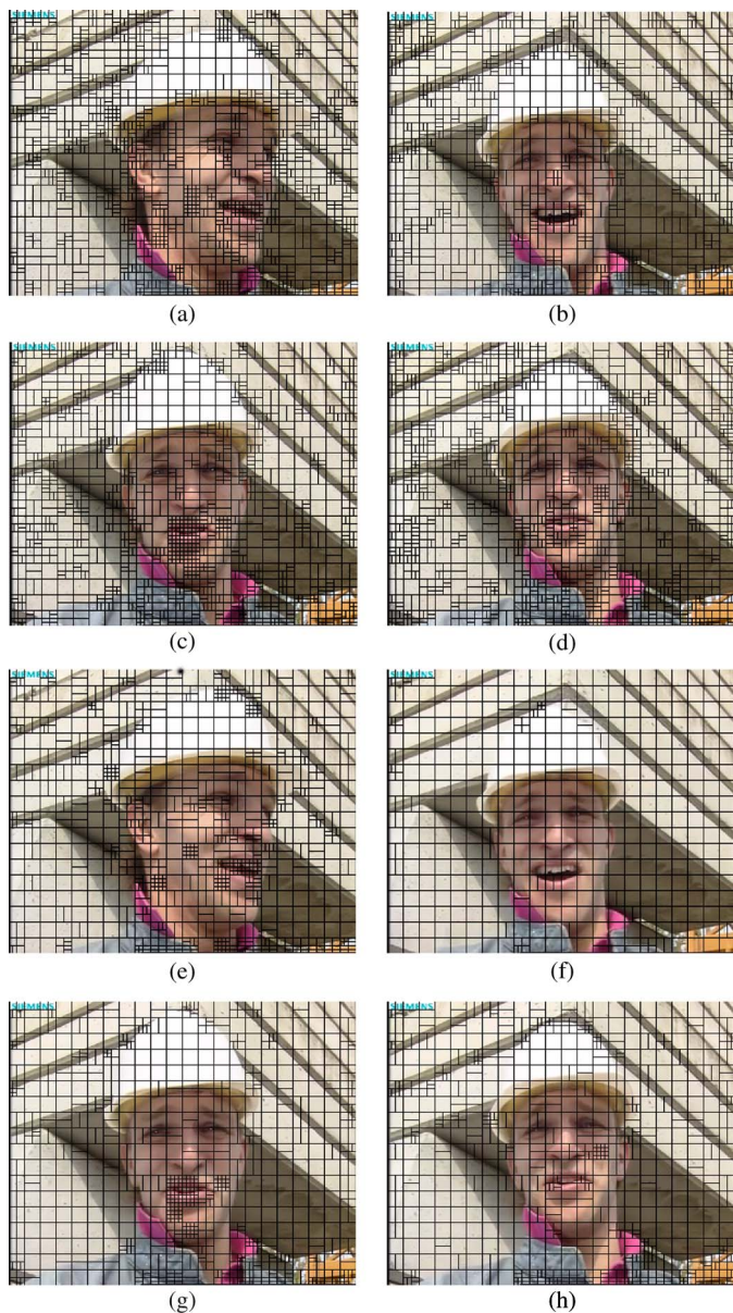
Fig. 5. Block partition of the 10th, 30th, 50th, and 60th frames of “Foreman” (CIF) [A bigger square grid represents a MB, a small one is the partitions of a MB; (a)–(d) is coded at 2 Mbps and (e)–(h) is at 500 kbps].
