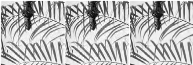
Fig. 4: Comparison of different methods at 0.35 bpp. Left: J2K (PSNR=24.29 dB, SSIM=0.8298); Middle: CADU (PSNR=24.62 dB, SSIM=0.8394); Right: WIDIC (PSNR=25.72 dB, SSIM=0.8878).
