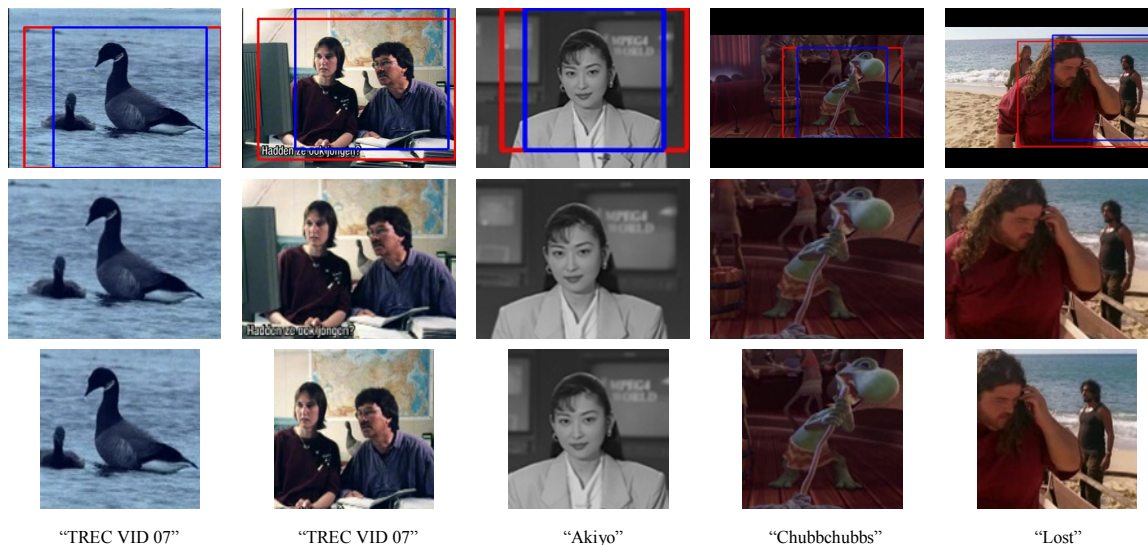
Fig. 11. Illustration of some retargeted results. The original frames scaled by adding letter box are shown in the first row. Results of the optimized cropping window trajectories for 160 \times 120 and 120 \times 120 target displays are marked with red and blue box respectively. The corresponding retargeted results are shown in the second and third rows. Our retargeting method zooms to the interest region in different scenes.
