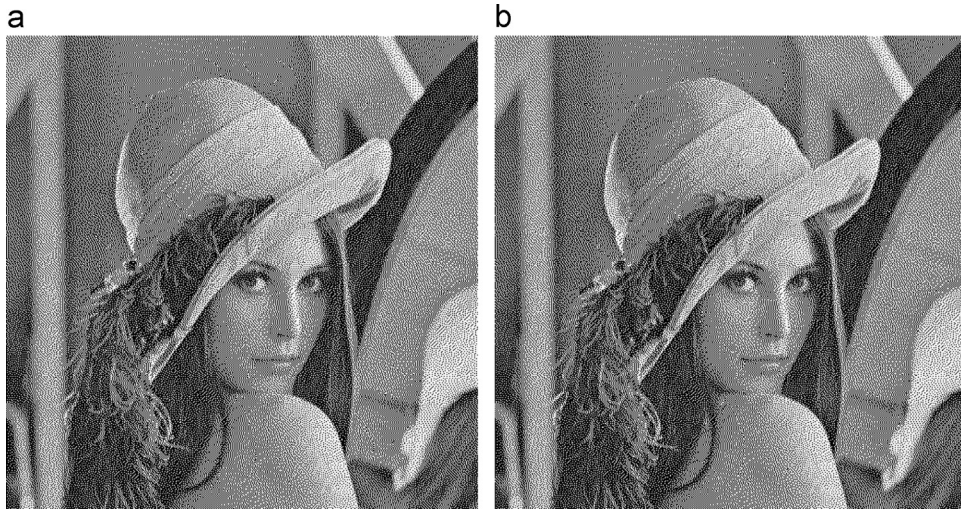
Fig. 20. (a) The to be printed DEED (L-2 Norm) Y_1, X_1 = X_2 , Steinberg kernel; (b) The to be printed DEED (L-2 Norm) Y_2, X_1 = X_2 , Steinberg kernel.
