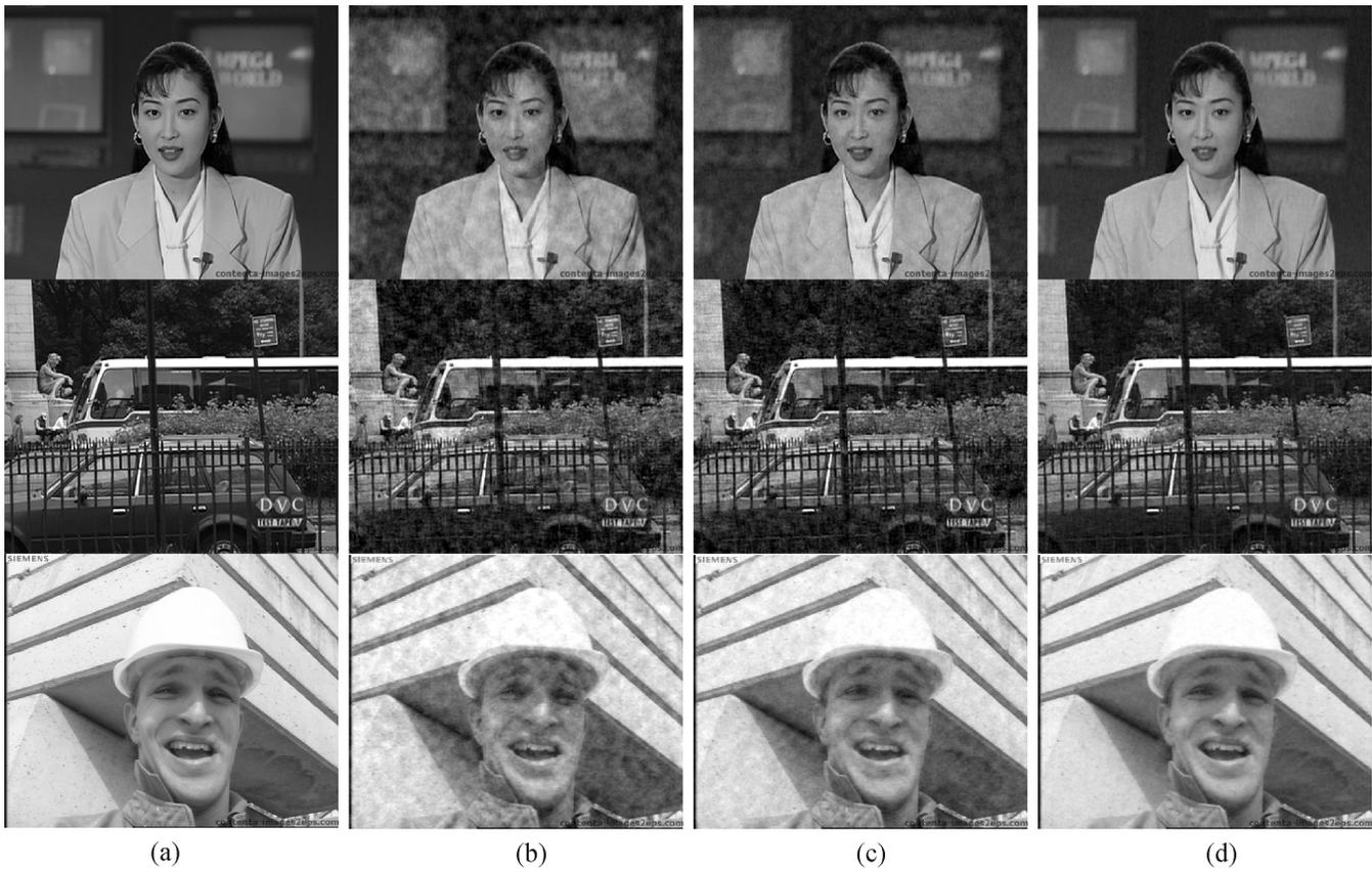
Fig. 12. Visual quality comparison, channel SNR is 5 dB. (a) Original frame. (b) Softcast2D. (c) Softcast3D. (d) DCast.
