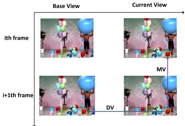
Fig. 1. Illustration of Disparity Vector (DV) and Motion Vector (MV).
