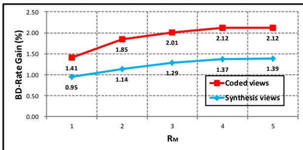
Fig. 6. Parameter  $R_M$  impact on the coding gains of coded views and synthesis views, respectively.
