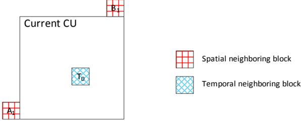
Fig. 2. Neighboring Blocks Disparity Vector (NBDV) scheme [10].
