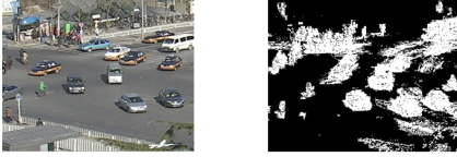
Fig. 3: (a) Original video of crossroad (cif) (b) Mask of result of subtraction of crossroad (cif), the black area is the background, the white area is the foreground
