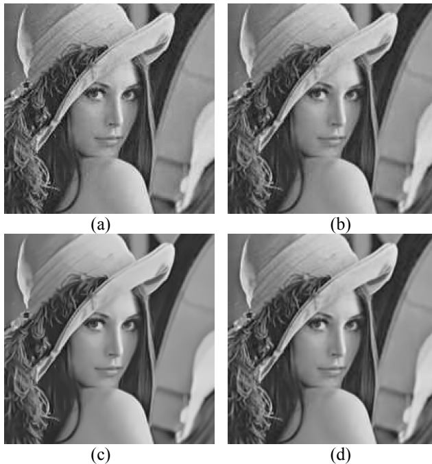
Fig.5: The reconstruction Lena with different methods ( QF=40 ), (a) JPEG decoder, (b) SPL [10], (c) NLM [13], (d) Proposed scheme.
