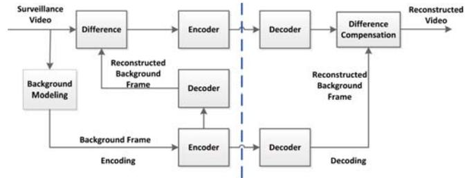
Fig. 1. The framework of background modeling based coding method
