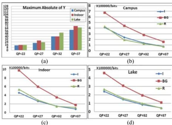
Fig. 4. (a) The maximum absolutes of Y component in residuals from sequences of Campus (blue), Indoor (red) and Lake (green); (b),(c),(d) Comparison of coding bits of I-frame with  $QP_{I-frame}$ , BG-frame with  $QP_{I-frame} - 10$  and maximum coding bits of Residual frame with  $QP_{I-frame} - 5$ ,  $QP_{I-frame} - 9$  or  $QP_{I-frame} - 11$
