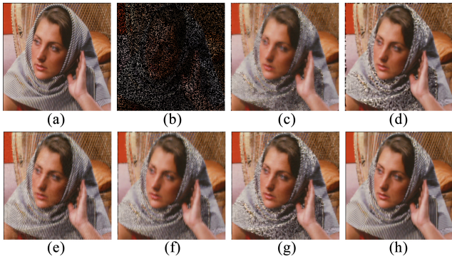
Fig. 8. Visual quality comparison of image restoration from partial random samples for image Barbara in the case of ratio = 20%. (a) Original image. (b) Degraded image with only 20% random samples available (7.36 dB/0.4998). (c)–(h) Restoration results by SALSA (22.75 dB/0.8193) [15], SKR (21.92 dB/0.8607) [35], MCA (25.69 dB/0.8939) [37], BPFA (25.70 dB/0.8927) [38], FoE (23.68 dB/0.8812) [36], and the proposed algorithm (27.54 dB/0.9264).
