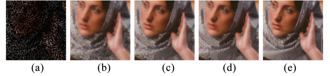
Fig. 4. Visual quality comparison of image restoration from partial random samples for crops of image Barbara in the case of ratio = 20%. (a) Degraded image with only 20% random samples available. (b) Restoration results by only local statistical modeling, i.e., LSM (22.18 dB). (c) Restoration results by LSM+NLM (22.97 dB). (d) Restoration results by NL/TV (23.08 dB). (e) Restoration results by LSM+NLSM, i.e., the proposed JSM (27.21 dB).
