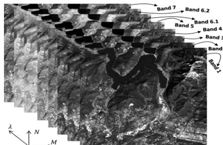
Figure 1. The 3-D structure of Landsat multispectral image.
