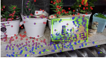
Fig. 3. The circles show local features, the green arrow line show the disparity of each local feature. The color of circles ranges from blue to red with the depth increase of local features. The target object is marked by a green bounding box.
