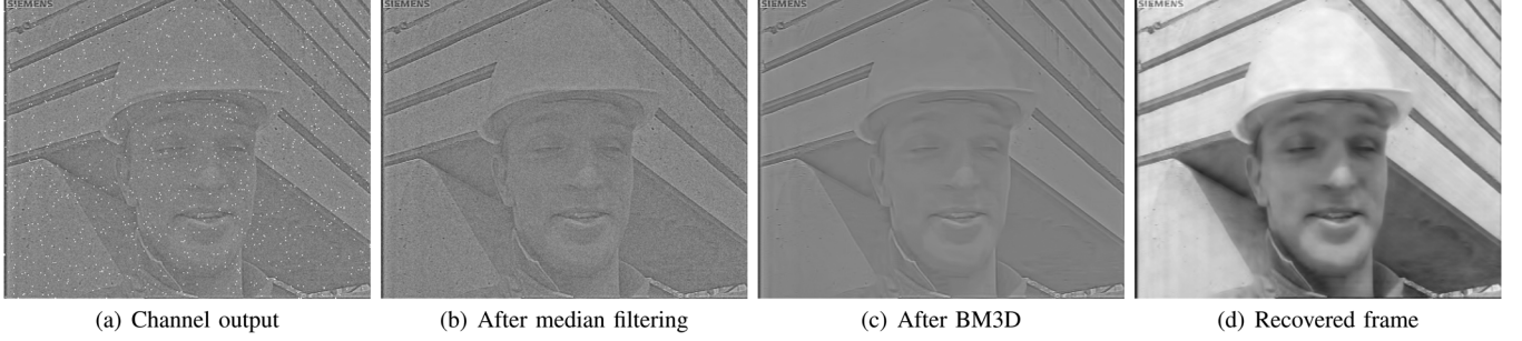
Fig. 3. Denoising processing at the receiver in the proposed framework. (a) Channel output; (b) After median filtering; (c) After BM3D; (d) Recovered frame.
