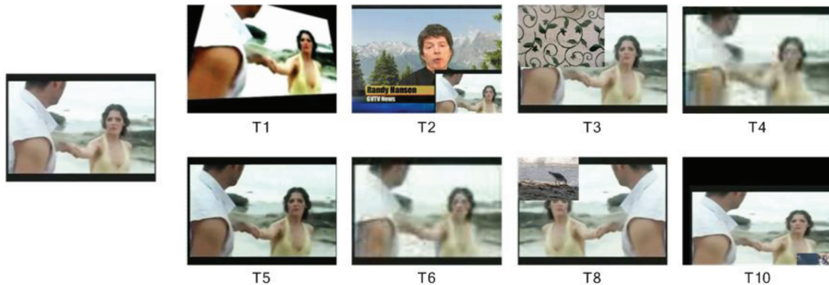
Fig. 1. Examples of video transformations. T1: camcording; T2: picture in picture; T3: insertion of pattern; T4: re-encoding; T5: change of gamma; T6: decrease in quality; T8: post production; T10: combination of 3 randomly chosen transformations. Note that T7 and T9 have been dropped by TRECVID 2010. Image courtesy Internet Archive [Internet Archive].
