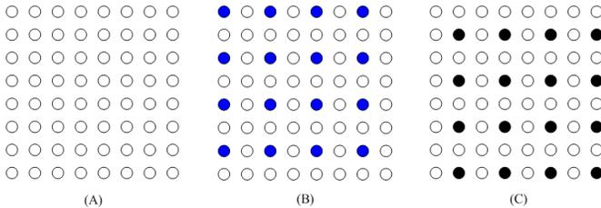
**Fig. 2.** Uniform downsampling with temporal multiplexing. (A) the original frame, (B) downsampled version (blue points) for odd frames; (C) downsampled version (black points) for even frames.
