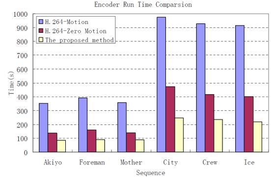
Fig. 5. Encoder complexity comparison
