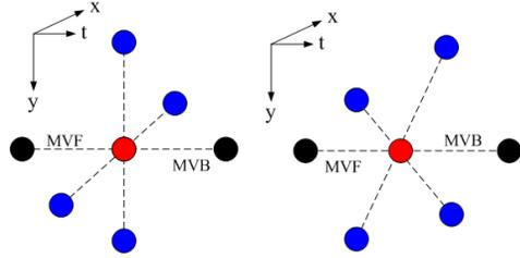
**Fig. 3.** Two used 6-order 3D-PAR model. The central pixel is in red, the spatial neighbors are in blue, and the temporal neighbors are in black which are aligned by MVs.
