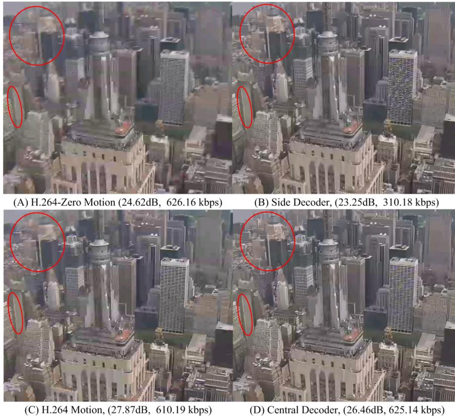
**Fig. 6.** Subjective quality comparison of reconstructed second frame in *City* sequence with (PSNR, Bit Rate) pairs.
