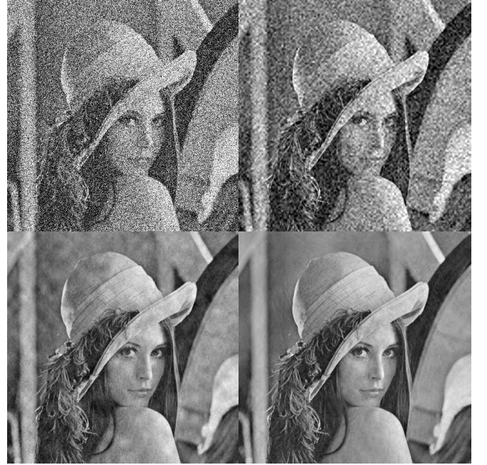
Fig. 10. Simulation results of SoftCast transmission using m -level DWT (CSNR= 4dB). From top-left to bottom-right: m = 0, 2, 4, 6 .
