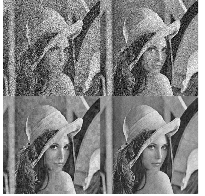
Fig. 9. Simulation results of SoftCast transmission using 2^m \times 2^m DCT (CSNR= 4dB). From top-left to bottom-right: m = 0, 2, 4, 6 .
