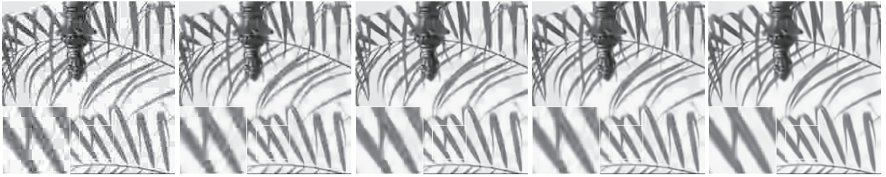
Fig. 1. Visual quality comparison of image deblocking for Leaves in the case of QF=5. From left to right: JPEG compressed image (PSNR=22.49dB; SSIM=0.7775), the deblocking results by Sun's [12] (PSNR=23.47dB; SSIM=0.8382), Foi's [18] (PSNR=24.28dB; SSIM=0.8653), Zhang's [14] (PSNR=24.13dB; SSIM=0.8548), and the proposed GSRQC (PSNR=25.11dB; SSIM=0.8865).
