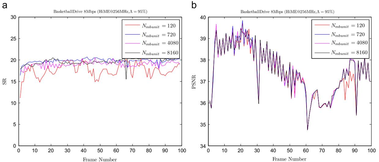
Fig. 7. Comparisons of CDSR with different sizes of BPU. (a) Search range comparisons for *BasketballDrive* 8 Mbps with HiME@256MHz and  $\Lambda_{TH} = 95\%$ . (b) PSNR curves for *BasketballDrive* 8 Mbps with HiME@256MHz and  $\Lambda_{TH} = 95\%$ .
