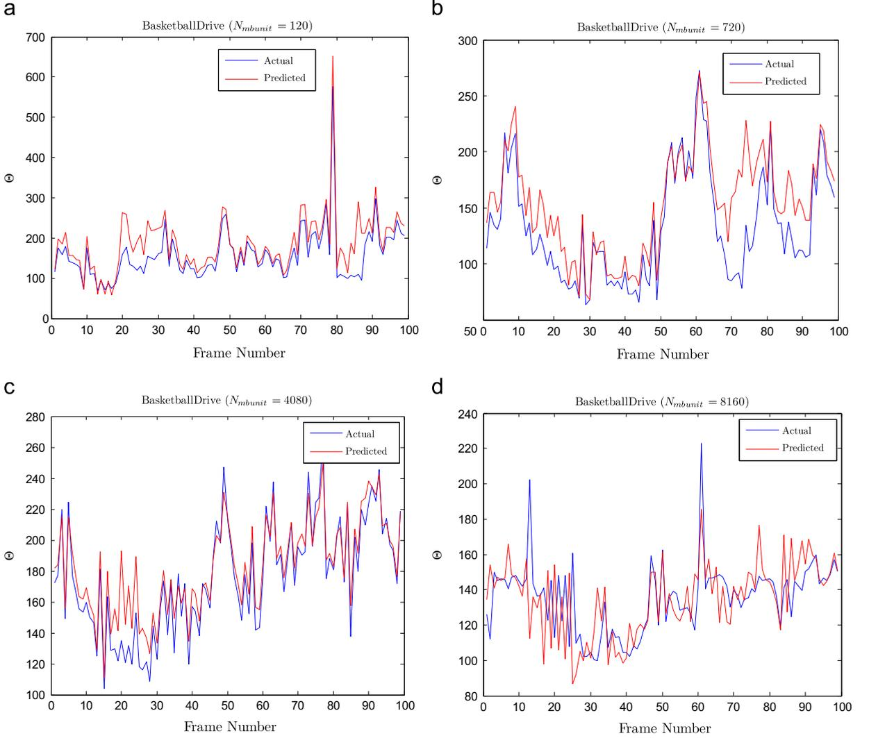
**Fig. 6.** Comparison of predicted and actual mean square of PMV deviations. (a) *BasketballDrive* with  $N_{mbunit} = 120$ . (b) *BasketballDrive* with  $N_{mbunit} = 720$ . (c) *BasketballDrive* with  $N_{mbunit} = 4080$ . (d) *BasketballDrive* with  $N_{mbunit} = 8160$ .
