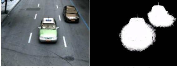
Original frame Initial mask Figure 3. Example of the initial mask in our method
