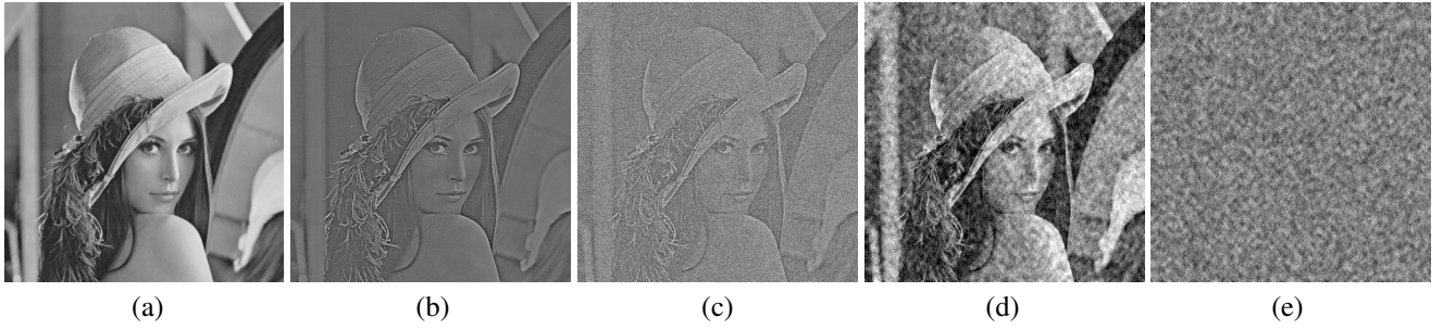
Fig. 2. An example of SoftCast transmission. (a) Original image, (b) Input to OFDM channel ( \{y_i\} shown in image domain), (c) Output from channel ( \{\hat{y}_i\} shown in image domain), (d) Image decoded by LLSE, (e) Reconstruction error in (d).
