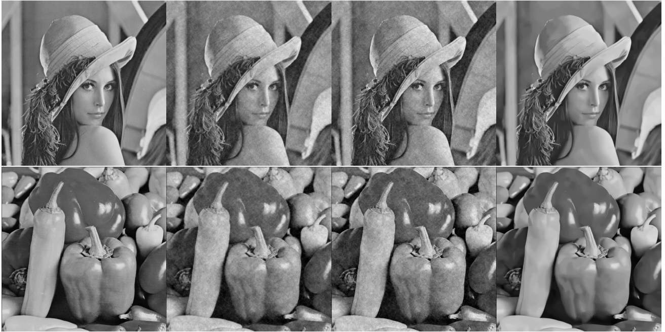
Fig. 4. Comparison of reconstruction images produced by different SoftCast reconstruction schemes (CSNR=2dB). From left to right: (a) Original image, (b) SoftCast+LLSE, (c) SoftCast+BM3D, (d) the proposed scheme. Enlarge the figure for details.
