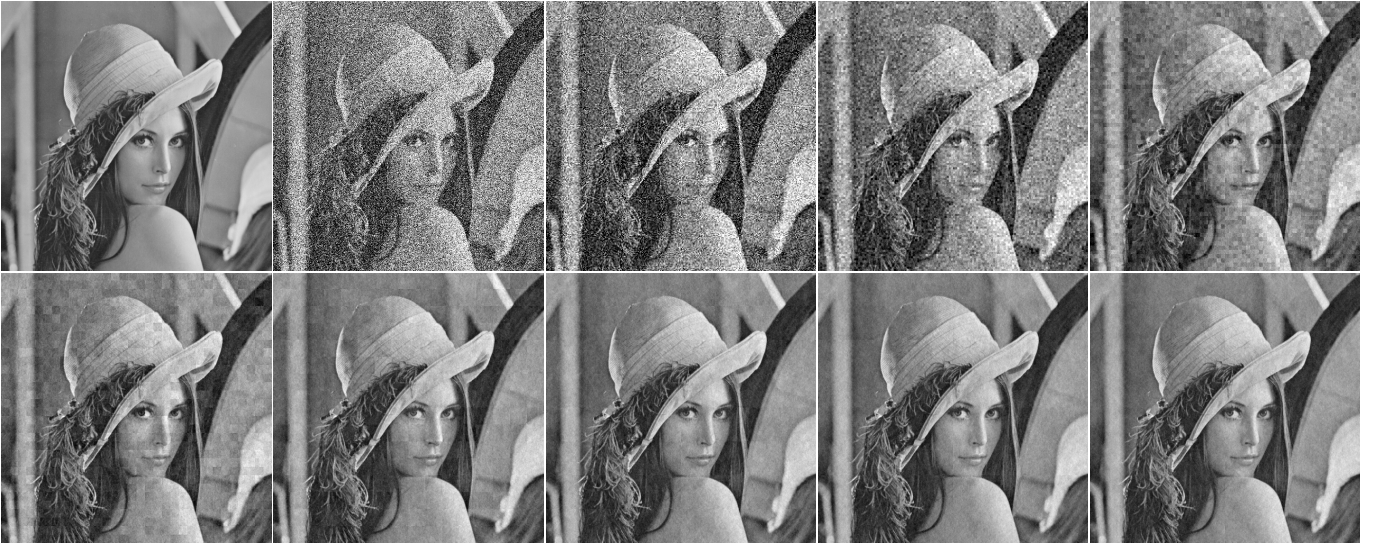
Fig. 10. The reconstructed images (of Lena ) in uncoded image transmission (with CSNR=4dB). From left (1 st row) to right (2 nd row): Original, DirectTx, Block-DCT with size 2^1 \times 2^1 , 2^2 \times 2^2 , 2^3 \times 2^3 , ..., 2^8 \times 2^8 . The PSNR goes from 11.09dB, 15.35dB to 31.45dB. Please enlarge the figure to observe details.
