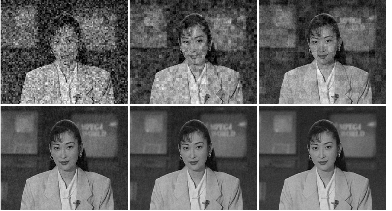
Fig. 14. The reconstructed frames (of Akiyo ) in uncoded video transmission (with CSNR=0dB). From left to right: GOP=1( 4 \times 4 ), GOP=1( 8 \times 8 ), GOP=1( 16 \times 16 ), GOP=1(Adaptive), GOP=2(Adaptive), GOP=32(Adaptive). Please enlarge the figure to observe details.
