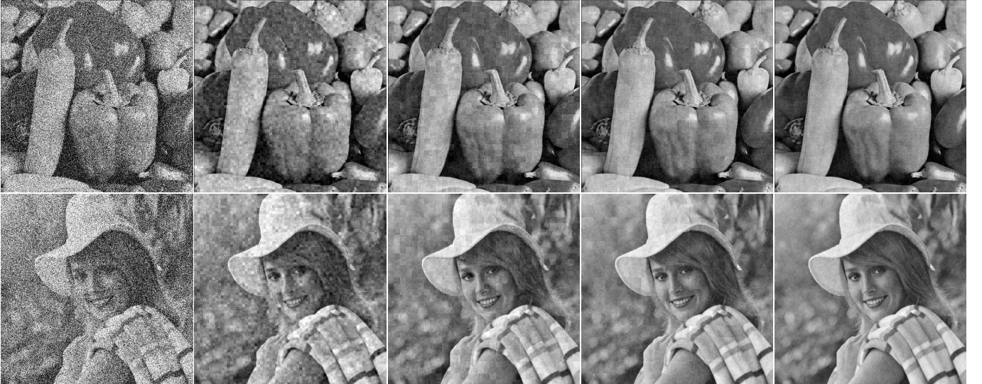
Fig. 11. The reconstructed images (of Peppers and Elaine ) in uncoded image transmission (with CSNR=4dB). From left to right: DirectTx, Block-DCT with size 2^3 \times 2^3 , 2^4 \times 2^4 , 2^5 \times 2^5 and 2^8 \times 2^8 . Please enlarge the figure to observe details.
