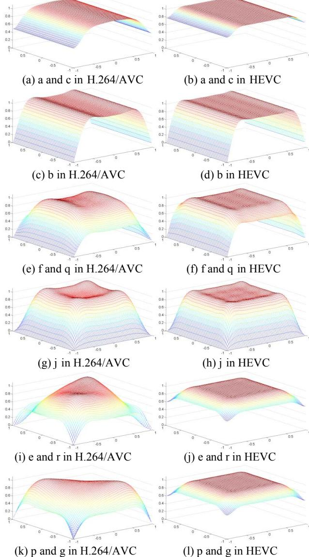
**Fig. 5.** Magnitude response curves of the interpolation filters in H.264/AVC and HEVC.
