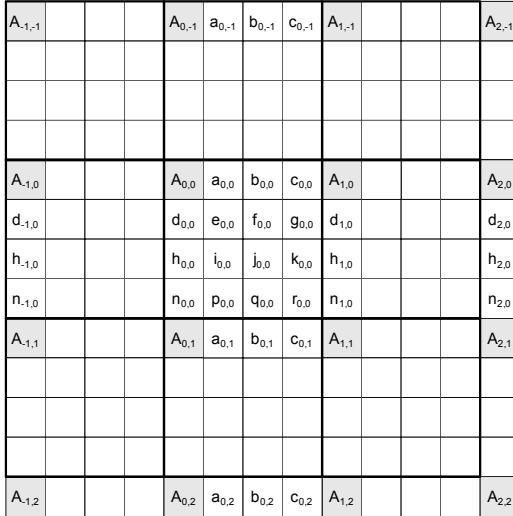
**Fig. 3.** Integer pixels (shaded blocks with upper-case letters) and fractional-pel pixels (un-shaded blocks with lower-case letters) for quarter-pel luma interpolation [11].
