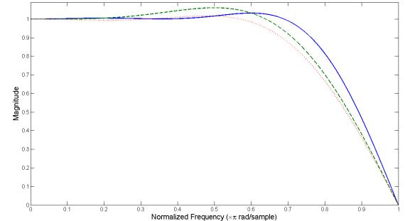
**Fig. 4.** Magnitude response curves of half-pel interpolation filters: DCTIF8 (solid), H.264/AVC (dashed), and DCTIF6 (dotted).
