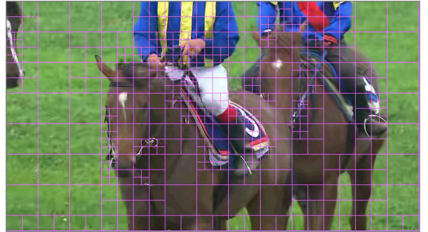
Fig. 1. The coding structure for a frame in RaceHorses with HEVC
