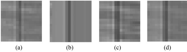
Fig. 3. An example of (a) luma block and its predictions by (b) AIP with mode 26; (c) ATMP; (d) CLNP.
