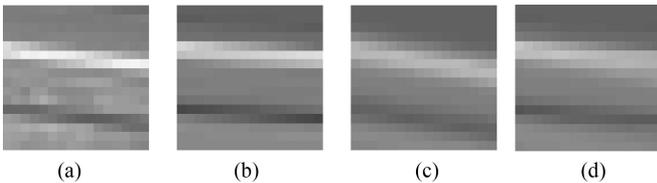
Fig. 4. An example of (a) luma block and its predictions by (b) AIP with mode 11; (c) AIP with mode 12; (d) CNMP with mode 11 and 12.
