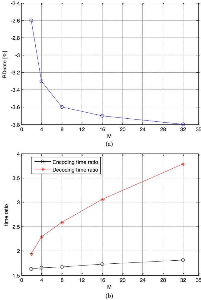
Fig. 9. The relations (a) between BD-rate reduction and  $M$ , and (b) between encoding/decoding time and  $M$ .
