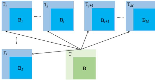
Fig. 6. Template matching process. Inverse-L shaped areas are the templates (in light blue and light green) used in the matching process. The deep blue blocks  $\mathbf{B}_1 \sim \mathbf{B}_M$  are the prediction candidates for the coding block  $\mathbf{B}$  (in green).
