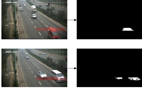
Figure 1. Two situations that need CCA and CNN. Images in the first row show that one vehicle is running across two lanes. Images in the second row show that two vehicles are running on their own lanes.
